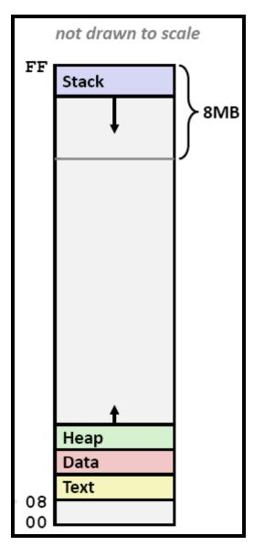
The stack starts very close to 0xFFFFFFFF (for 32-bit) and grows DOWN
