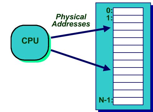
Addresses generated by the CPU correspond directly to bytes in physical memory
